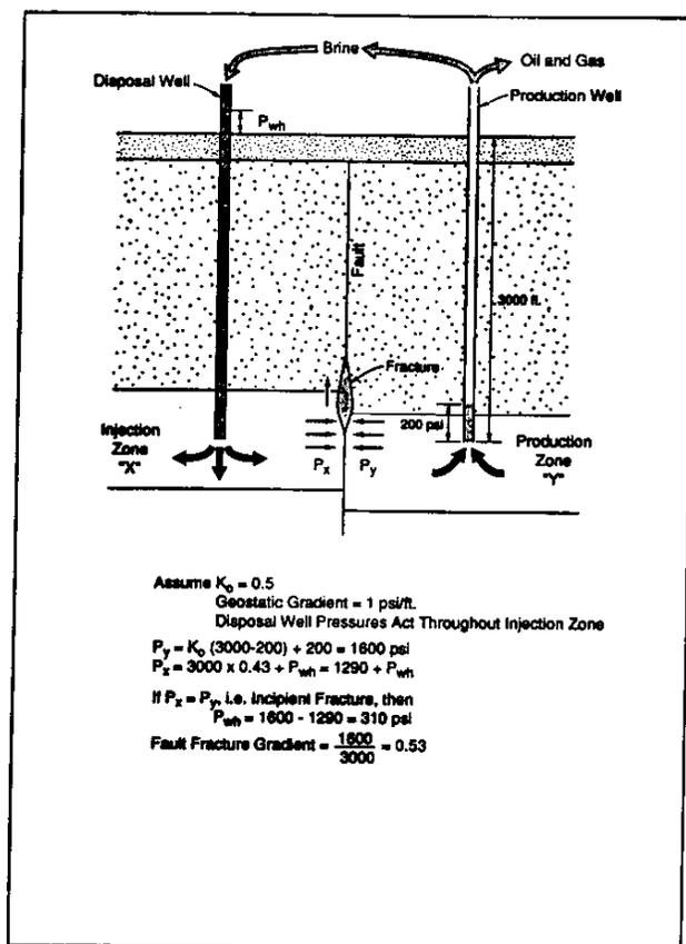
Figure 9. Fault injection pressure for case of long term injection
