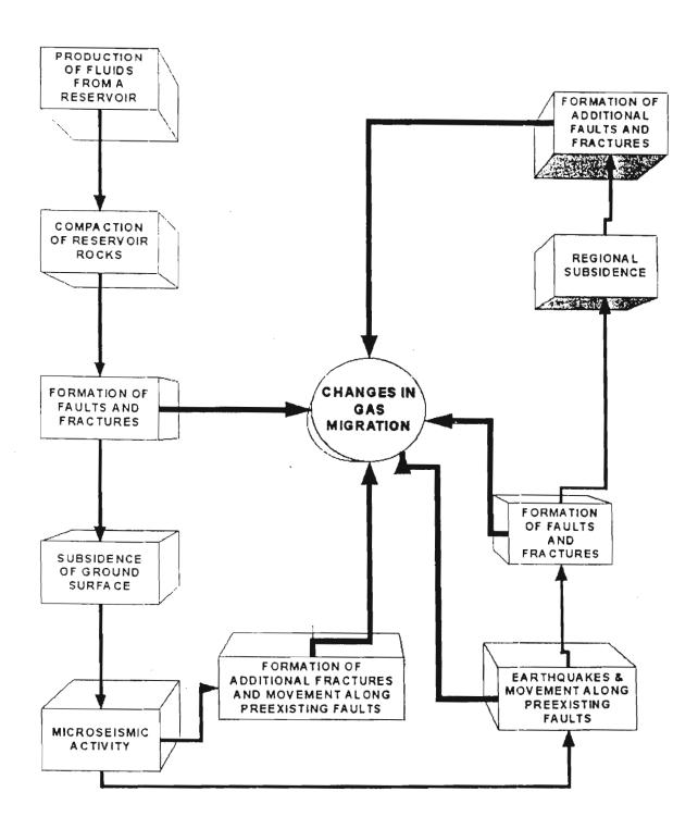
Figure 1. Schematic diagram of system relationships among the production of fluids, compaction, subsidence, and seismic activity. (Modified after Chilingarian et al., 1995, fig. 1, p. 41.)
